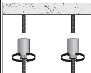
Step 1 Thread couplers onto assembly
