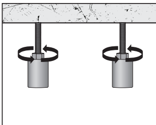
Step 1 Thread couplers onto hanging rod
