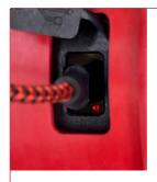
The LED is **Red** when the battery is charging.
