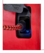
And is **Blue** when the battery is fully charged.
