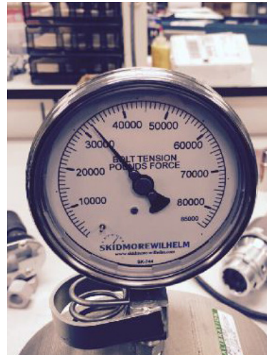
Minimum of 28 kips required per manufacturer specifications
