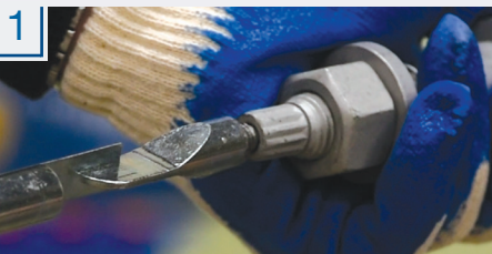
1 Thread the installation tool tip into the splined end of the bolt.
