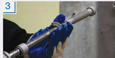
3 Move the collapsible washer to the correct location on the tool and fold in place.
