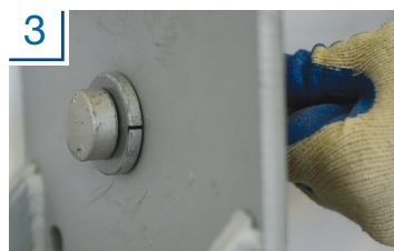
3 Pulling back, rock the tool side-to-side to engage the collapsible washer.
