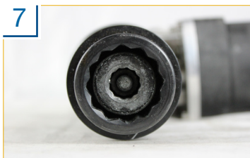
7 Using the shear wrench engage the outer socket with the splined end of the bolt. Press the trigger until correct tension has been achieved (the bolt spline separates from the bolt).
