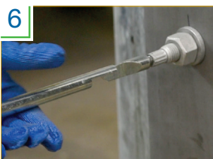
6 Remove the tool by unscrewing it from bolt (counterclockwise).
