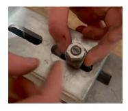
**2.** Insert the T-bolt into the slots, with the vertical line still parallel.
